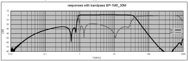
Transmission and input return loss with 1 ... 30 MHz band pass filter BP-1M0\_30M installed in RF input.
