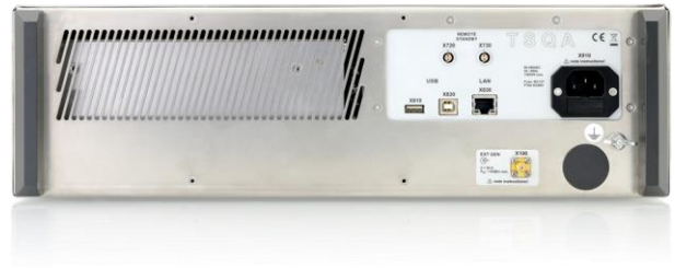
TSQA-1X8PF with RF ports and power/remote (Similar appearance)
