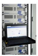
Appearance: Option drawer with control PC mounted in 19" system rack.
