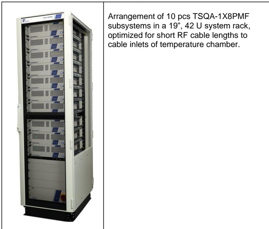
Arrangement of 10 pcs TSQA-1X8PMF subsystems in a 19", 42 U system rack, optimized for short RF cable lengths to cable inlets of temperature chamber.
