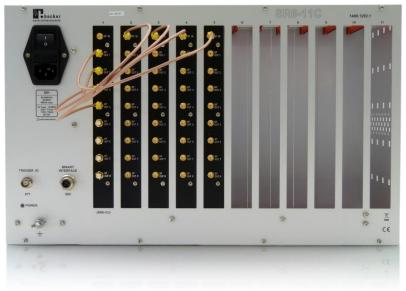
Rear view shows WSDU-1X32 wideband signal distribution equipped with RF cables in the 1X32 configuration. Unused outputs are terminated by 50 ohm SMA resistors. (Located on the lower section of module on the left side).
