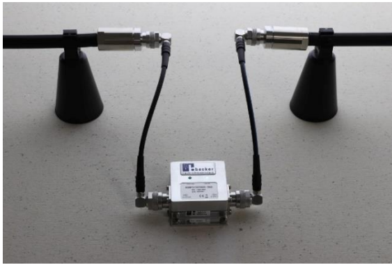
Figure 5: inline Wi-Fi booster installation example
