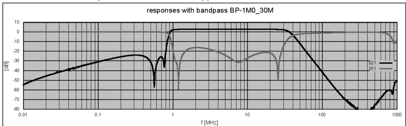
Transmission and input return loss with 1 ... 30 MHz band pass filter BP-1M0\_30M installed in RF input.
