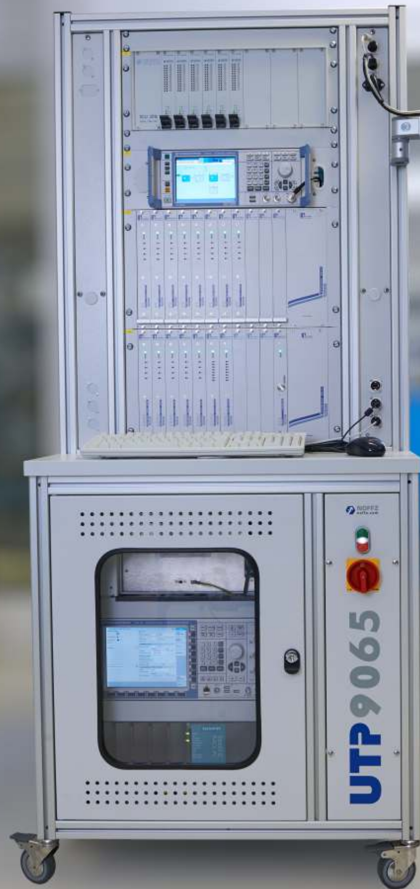
Courtesy to Noffz Technologies GmbH. Complete test system for validation of infotainment and connectivity modules in the car.
