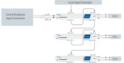
Cascading RSDU-2X4AR devices causes slightly increasing noise and decreasing dynamic range performance (approx. 1 dB per section).
