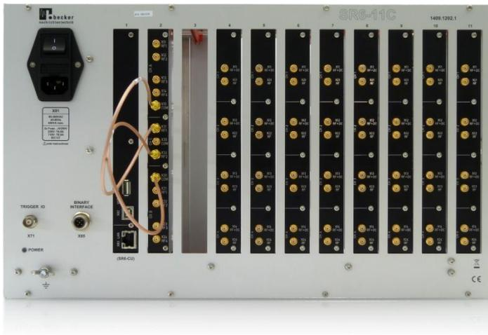
Rear view shows RSWU-2SP4TS+ switch with RF cables for SP8T "1X8" configuration
